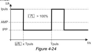
AMP = Main current; e.g. 100 A IPL = Pulse current = IP1 x AMP; e.g. 170% x 100 A = 170 A IPP = Pulse pause current Tpuls = Duration of one pulse cycle = 1/FrE; e.g. 1/1 Hz = 1 s bAL = Balance**Selection**
