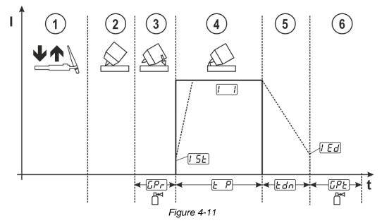
As an example the process is shown with HF ignition. Arc ignition with lift arc is also possible, however > see 4.1.3 chapter.
