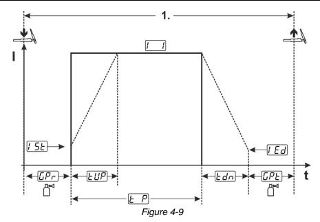
As an example the process is shown with HF ignition. Arc ignition with lift arc is also possible, however > see 4.1.3 chapter.
